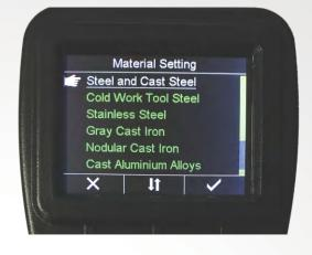
The HT-10 has build in data logger with capacity to store measurements. The data can be transferred via USB 2.0 communication port to PC and a quick report with ease can be generated within no time through <u>Datapro Software</u>. Complete data of hardness values, average values, material, impact directions, date & time of measurement are all captured and stored through which a statistics analysis can be performed.
